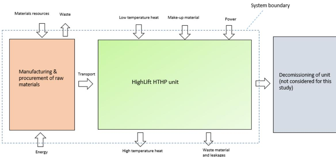
Figure 8. Schematic diagram of the system boundary for life cycle assessment of HTHP.
