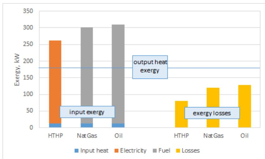
Figure 6. Exergy inputs, output and losses for a 250 kW 180 °C heat output system using a heat pump, natural gas-fired boiler or oil-fired boiler.
