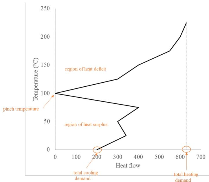
Figure 5. An example of a Grand Composite Curve. From the graph the total heating and cooling demand for the process and temperature regions of heat surplus and deficit. The temperature dividing the regions is called the 'pinch temperature'.
